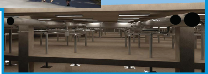
Rendering of the intersitial building systems floor. Courtesy of HKS Architects
